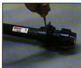
5. Use chain wrench to fastened the Locking Nut.
